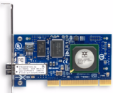
32-bit PCI-X connector
