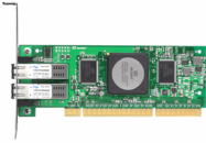
64-bit PCI-X 2.0 connector
